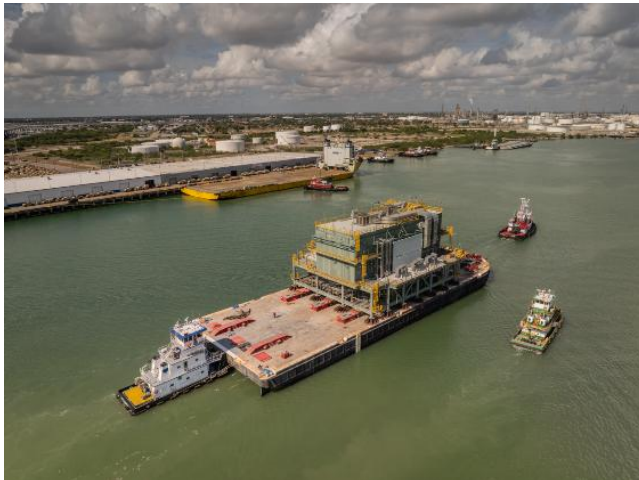
CAPTION: Transport of the 1,334 MT module, measuring 38.3 x 31.6 x 21.3 m, from Port Ingleside, Texas, to the Port of Corpus Christi, Texas, USA
