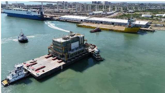
CAPTION: Arrival of the 1,334 MT module, measuring 38.3 x 31.6 x 21.3 m, at the Port of Corpus Christi, Texas, USA
