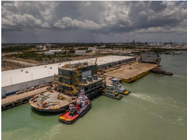
CAPTION: Arrival of the 1,334 MT module, measuring 38.3 x 31.6 x 21.3 m, at the Port of Corpus Christi, Texas, USA
