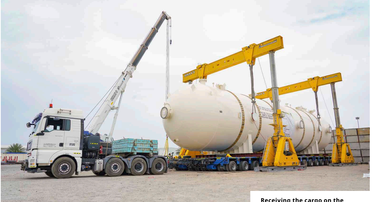
Receiving the cargo on the multi-axle hydraulic trailer
