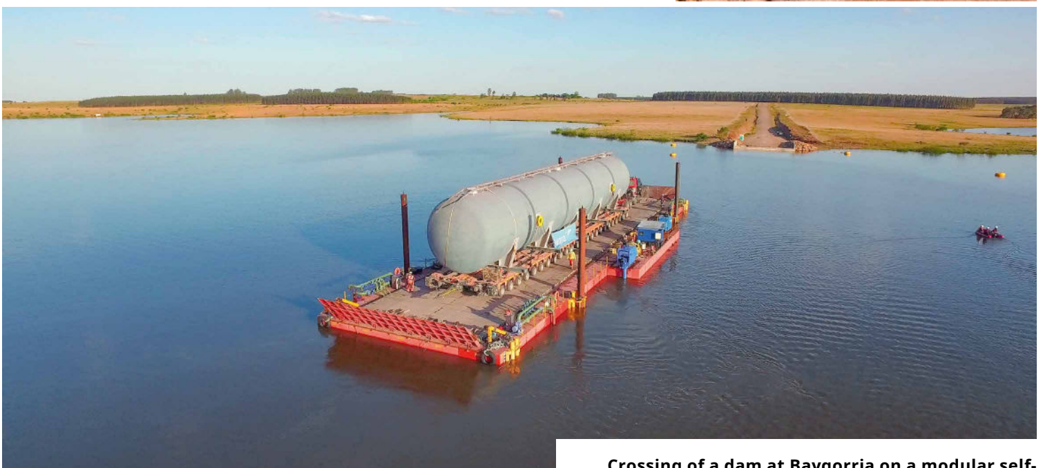
Crossing of a dam at Baygorria on a modular self-propelled barge exclusively designed for the project
