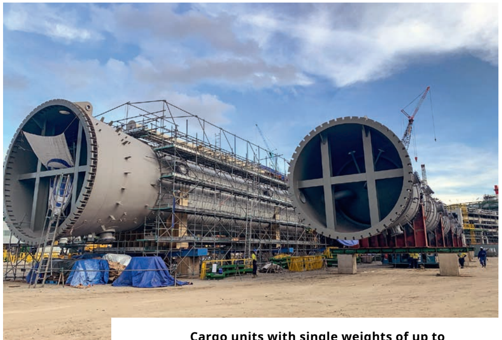
Cargo units with single weights of up to 778 metric tons and lengths of nearly 100 meters
