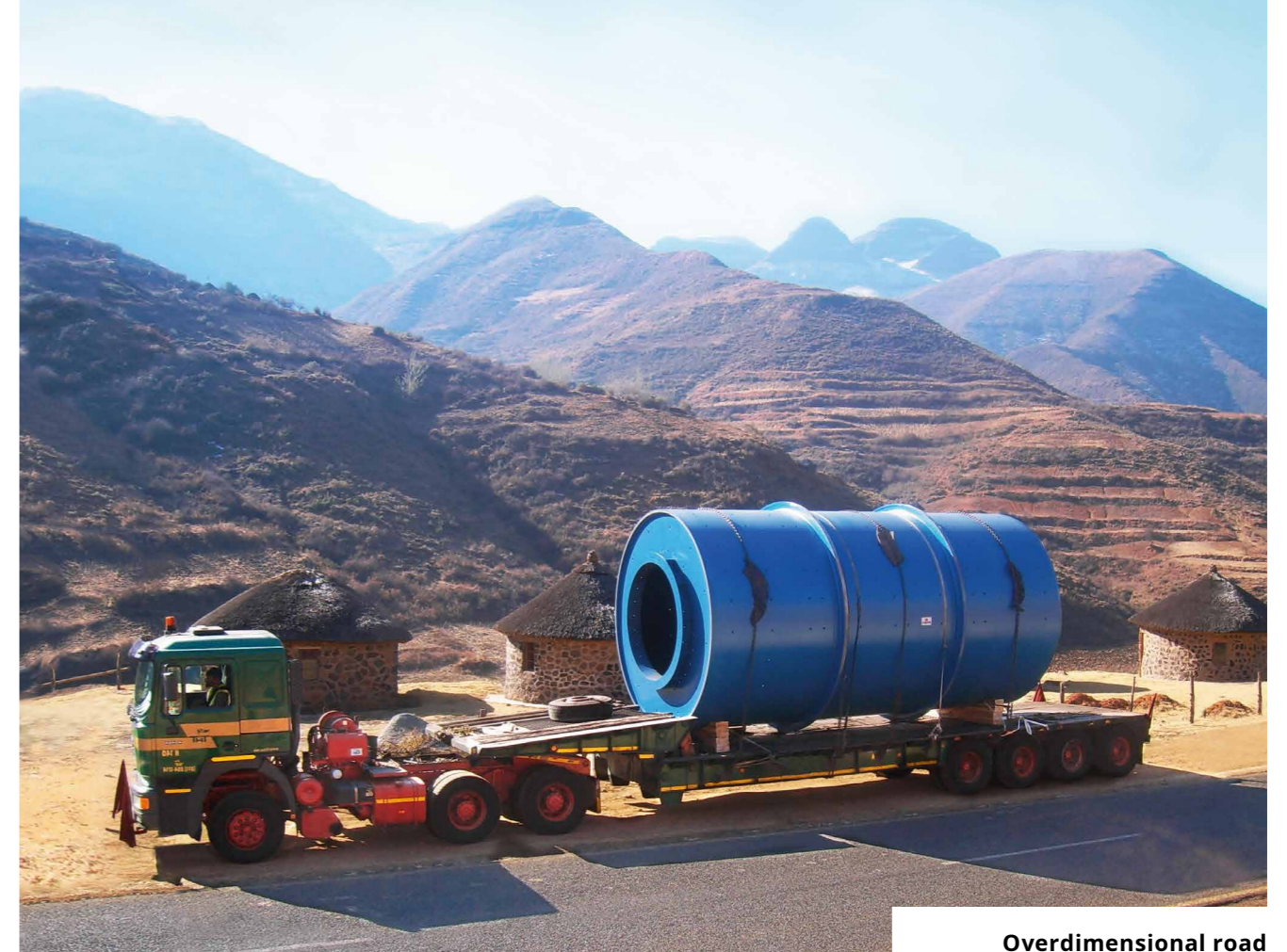
Overdimensional road transportation of a scrubber drum for the Letseng Diamonds Project
