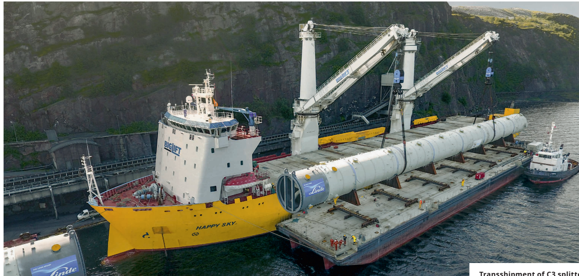
Transshipment of C3 splitter onto barges in the remote area of Kirkenes, Norway
