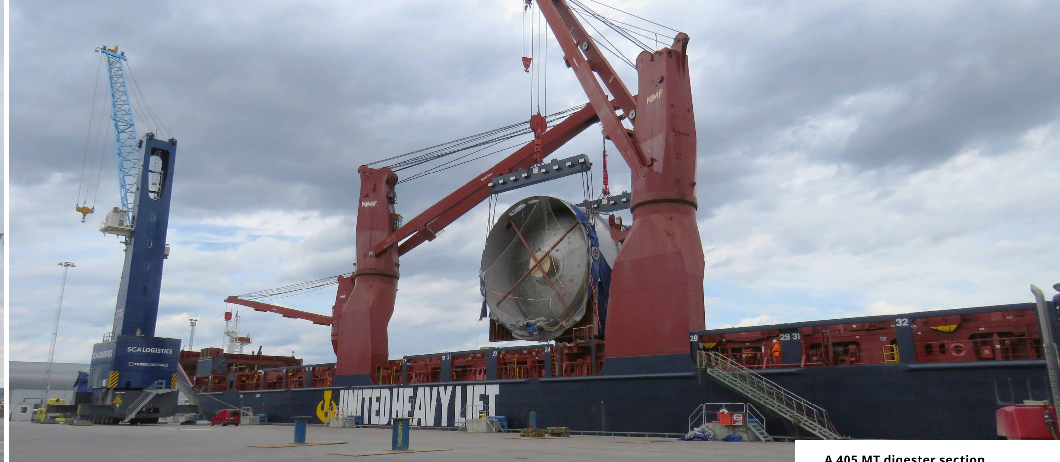
A 405 MT digester section being lifted by vessel gears in Port Tunadal
