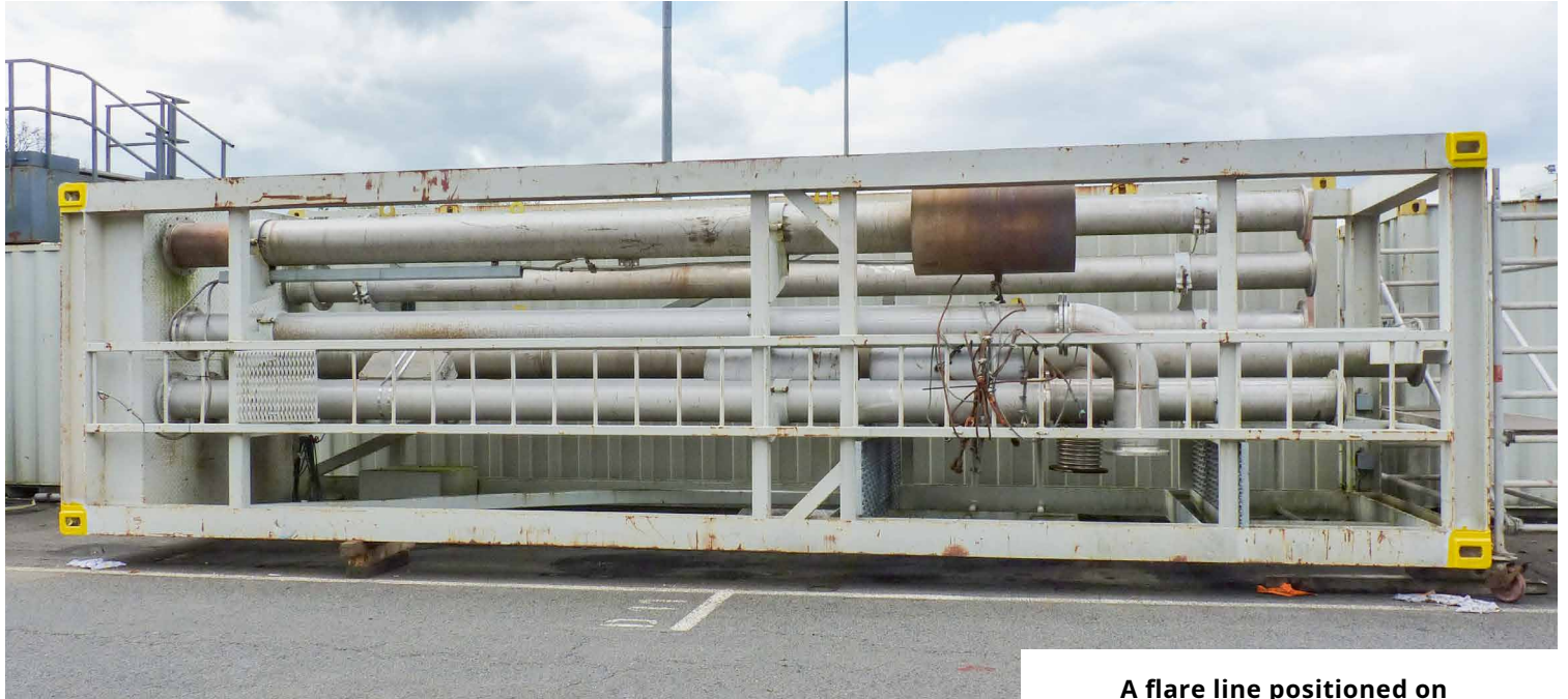
A flare line positioned on beams at the production site, ready for its transportation
