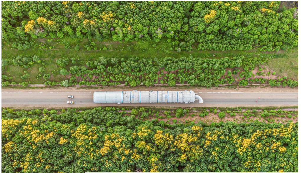
Primary fractionator on its way to the job site
