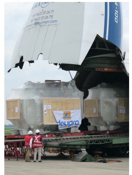
Both transformers on the ramp, ready for offloading
