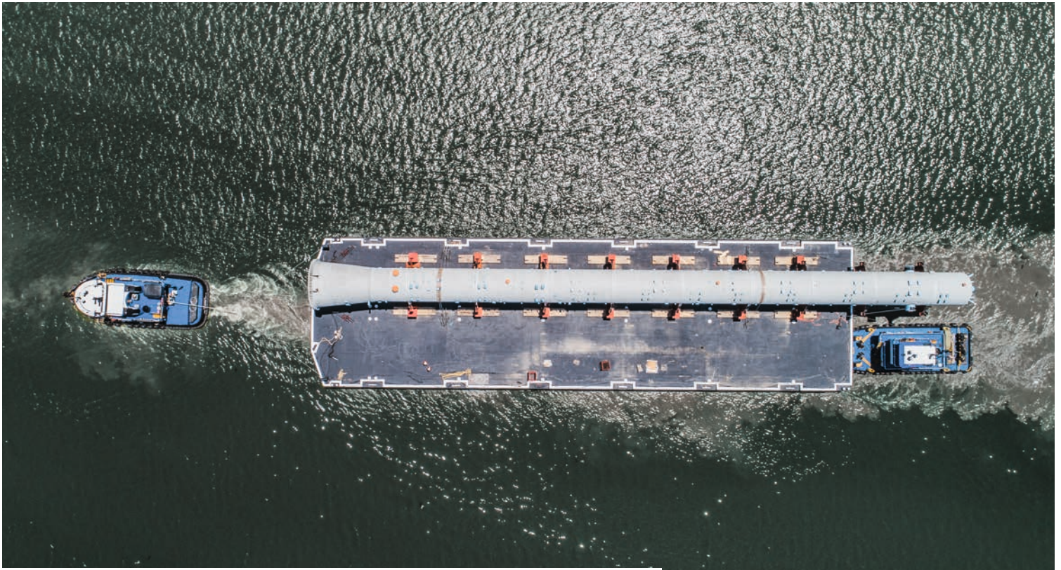
Barge voyage through Buffalo Bayou to Scott Bay showing the C6 column hanging over of the barge's stern by approximately 20 m
