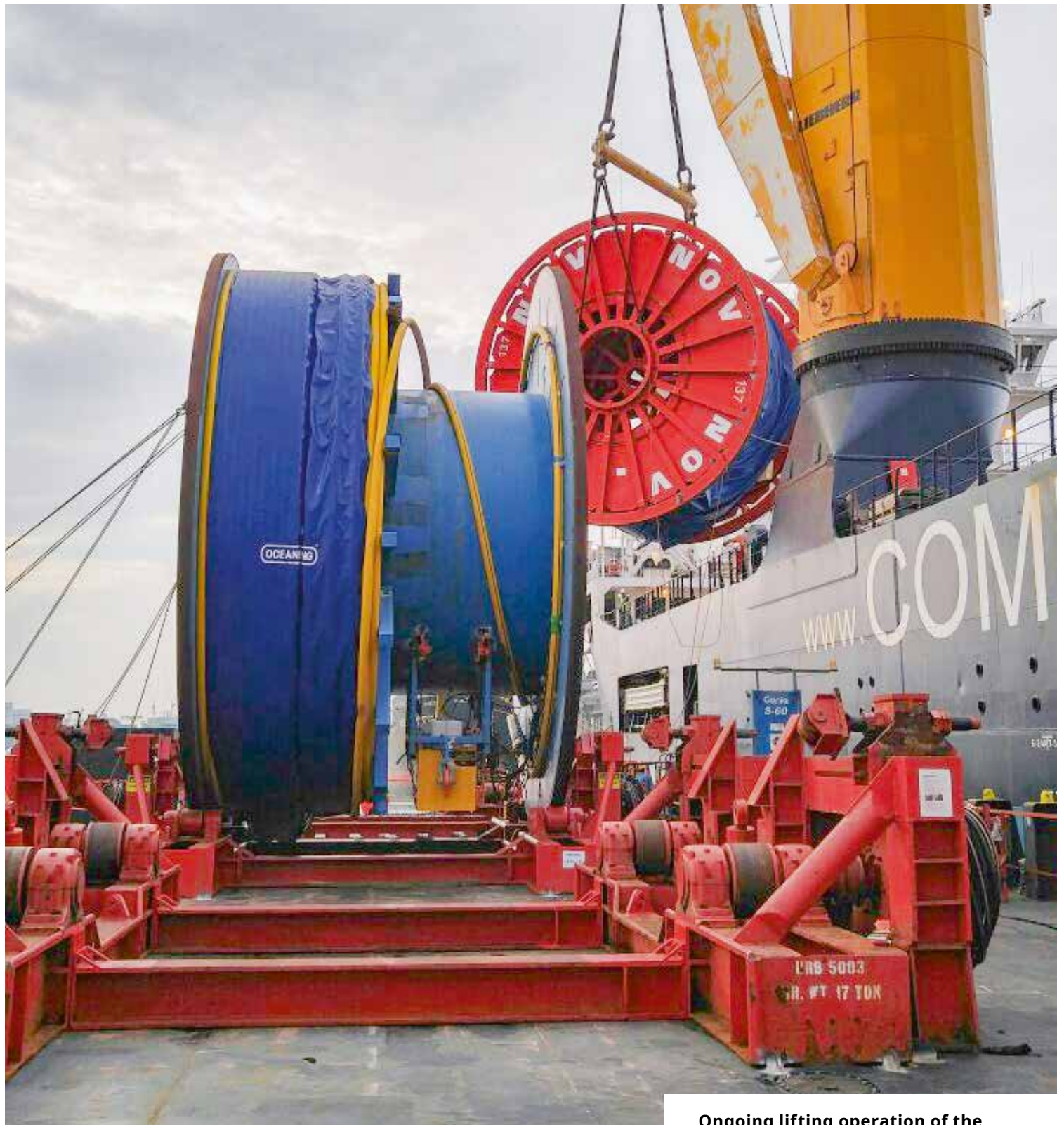
Ongoing lifting operation of the 245 MT flowline reel: The 205 MT umbilical reel (blue) is sitting safely and securely on the pre-fitted reel-powered under roller.
