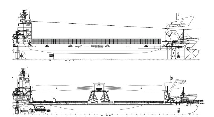
rotor blades. The vessel is assigned to navigate between production facilities in the UK, Denmark and Germany and their respective installation harbors. In 2021 and 2022, the vessels went to the shipyard for modification. Rotra Mare will become wider and longer to feature an overall length of 152.70 meters. This will enable the vessel to transport 12 blades with a maximum length of 97 meters or nine blades of 108 meters in length.
