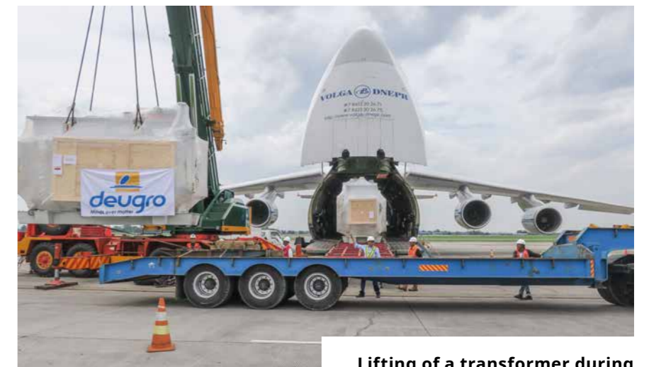
Lifting of a transformer during offloading operations in Medan, Indonesia
