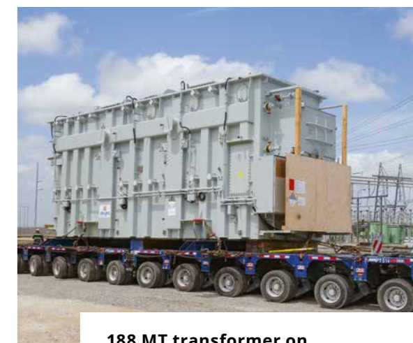
188 MT transformer on its way to a substation in Texas, USA
