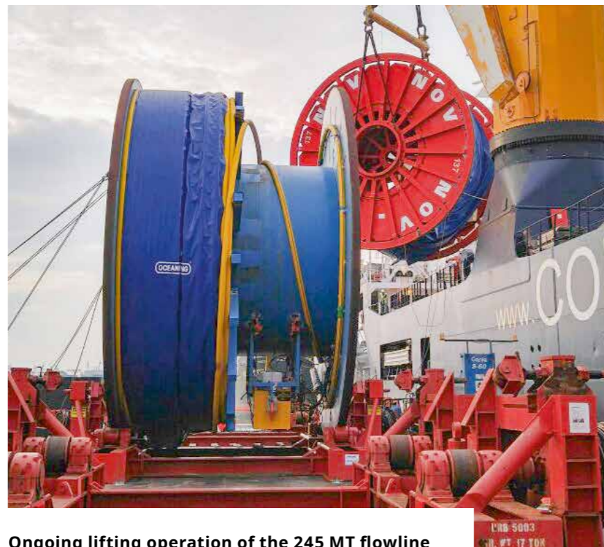
Ongoing lifting operation of the 245 MT flowline reel: The 205 MT umbilical reel (blue) is sitting safely and securely on the pre-fitted reel-powered under roller.
