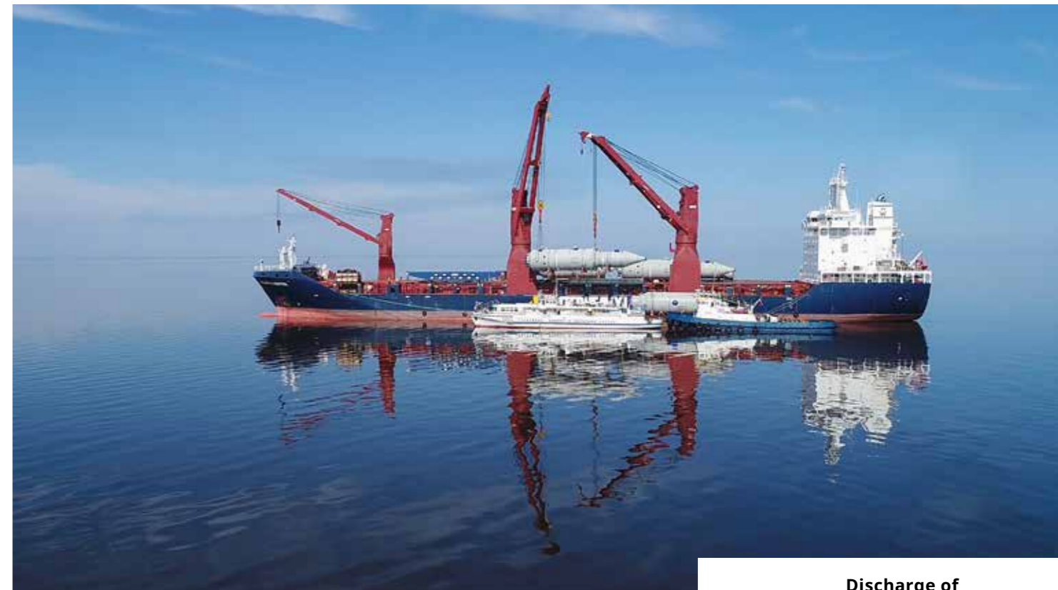
Discharge of oversized cargo at anchorage at Novy Port
